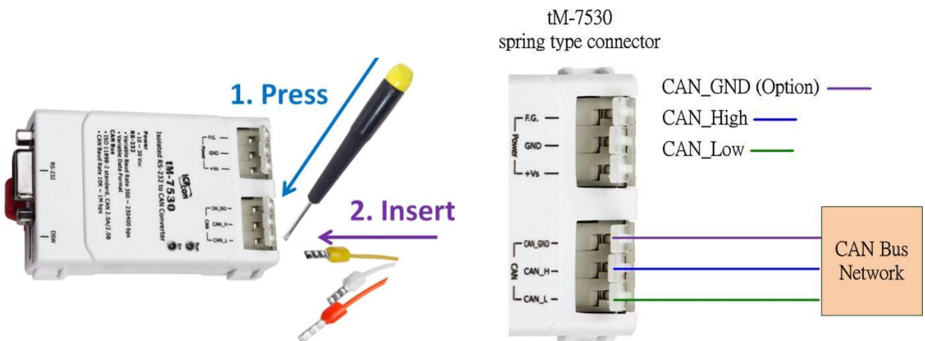
Figure: tM-7530 CAN bus wiring method
