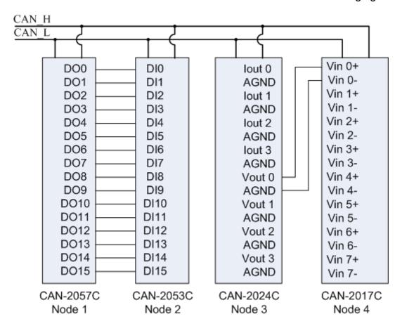
Please use rotary switch to set the node ID from 1 to 4, and CAN bus baud rate to 125Kbps. Moreover, refer to manuals of these modules to set the CAN-2024C and CAN-2017C input/output range to -10V~+10V. The four modules' information is as below.
