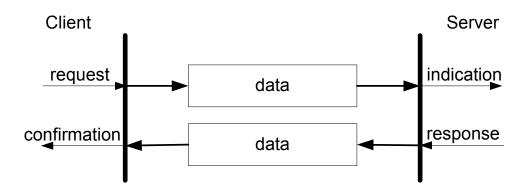
The SDO has two kinds of the COB-IDs, RxSDOs and TxSDOs. They can be viewed in the CANopen device. For example, users send a SDO message to the CAN-2000C modules by using RxSDO. On the contrary, the devices CAN-2000C transmit a SDO message by using TxSDOS.
