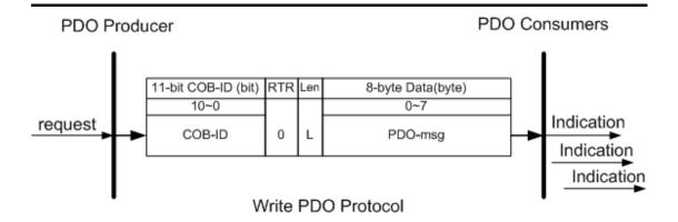
**COB-ID**: the default PDO COB-ID, or the PDO COB-ID can be defined by
