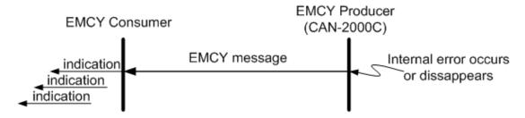
An emergency message containing 8-byte of data is called emergency object data. The abbreviated diagram is shown below, and all fields in the emergency object data will be described in section 5.3.
