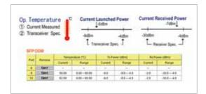
The JetNet 6059G SFP socket supports 100Base-FX single-mode/multi-mode and 1000 Base-FX single-mode/multi-mode transceiver with speed detection and independent indication. Moreover, it supports DDM (Digital Diagnostic Monitoring) type SFP transceivers allowing users to diagnose optical cable transmission problem through maintenance and debugging of the optical signal quality by DDM without the need of an extra optical cable analyzer, as a result greatly saving time and system costs.
