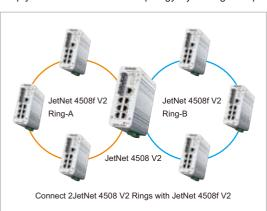
rings into a line or into multiple directions. In addition to extensibility, MultiRing<sup>TM</sup> has great diversity of various ring technologies. When MultiRing<sup>TM</sup> enabled, JetNet 4508f V2 can connect RSR rings, TrunkRing<sup>TM</sup> and a Super Ring together and simultaneously provide more Fast Ethernet Ring connectivities. This provides extensibility to new technologies while keeping the great backward compatibility.
