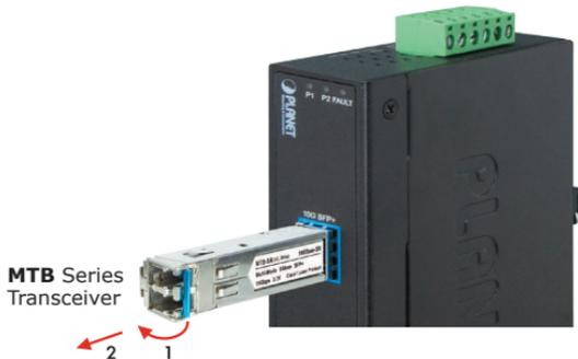
Figure 3-2: Pulling Out from the Transceiver
