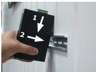
**Step 3:** Make sure the DIN rail is tightly secured on the track.
