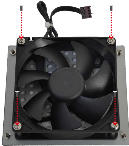
Figure 3-5: System Fan Installation
