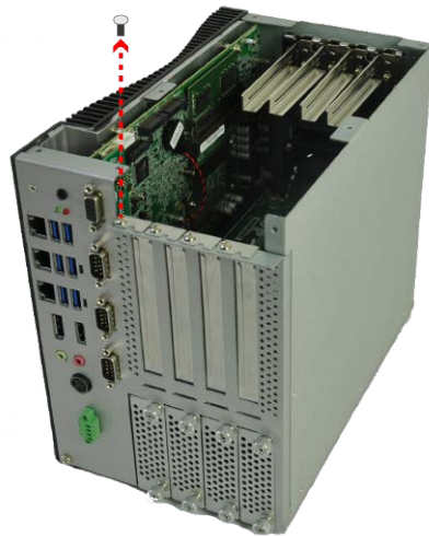
Figure 3-20: Remove Expansion Slot Bracket
