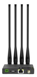
UF31 is a high-performance 5G modem for 5G wireless networking applications. It supports 5G NSA&SA, 4G LTE and 3G networks from telecom service providers of most countries in the world. The USB type-C port and Ethernet port are adopted to provide high-speed internet access for field devices.
