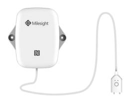
EM300-SLD is a compact spot leakage detection sensor for detecting presence of water (or other liquids) and transmitting alarm using LoRaWAN® technology. With this low power consumption technology, EM300-SLD can work up to 5 years with 4000 mAh battery. Combining with Milesight LoRaWAN® gateway and Milesight IoT Cloud solution, users can manage all sensor data remotely and visually and receive alarms via mobile APP.
