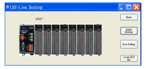
**Step 5:** Then, repeat the step 3~4 to configure the slot 1 to I-8042 module. Then, click "Save Setting" button to finish the off-line parameter settings..
