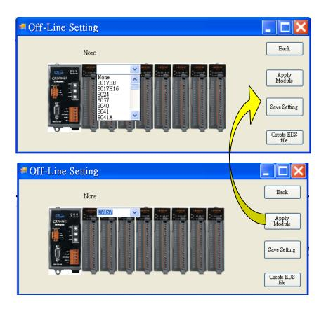
**Step 4:** After finishing the configuration, users can one-left click on the slot module in the "Off Line Setting" frame if need to change the configuration. If the configuration is successful, users can see the correct module name when mouse moving in, for example 87057 on the top of the slot module.
