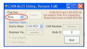
**Step 2:** Take the CAN slave device (CAN-8823 with node ID 1) as an example, Users have to fill in "NODE ID" with 1 and choose "Device Name" with CAN-8823. Then, press "Next" button.
