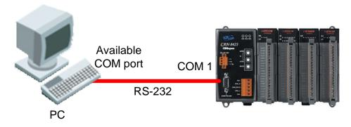
**Step 1:** Turn off the CAN-8423. Set the "Baud" rotary switch of CAN-8423 to 9 for configuration mode. Then Turn on the CAN-8423.
