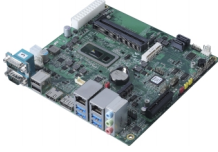
1 x LV-67Z Mini-ITX Motherboard (include Cooler Fan)
