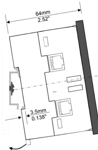
Figure 5. Snapping the Controller on to the DIN Rail
