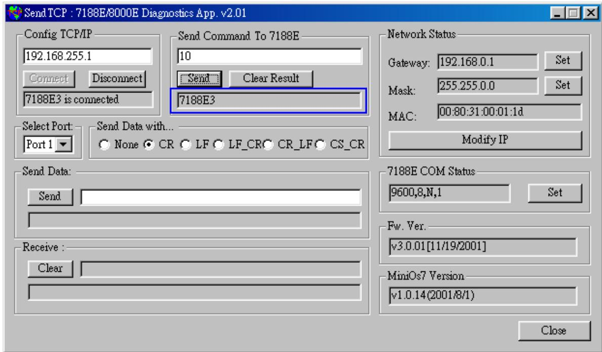
Step 4: Select “Port 2” and “CR”. Then send “\$02M” to read 7000 module’s ID which is connected to I-7540D’s COM2. If you enable 7000 module’s checksum function, select “CS\_CR”. The “CS\_CR” option will add two checksum bytes, then adds “CR”.
