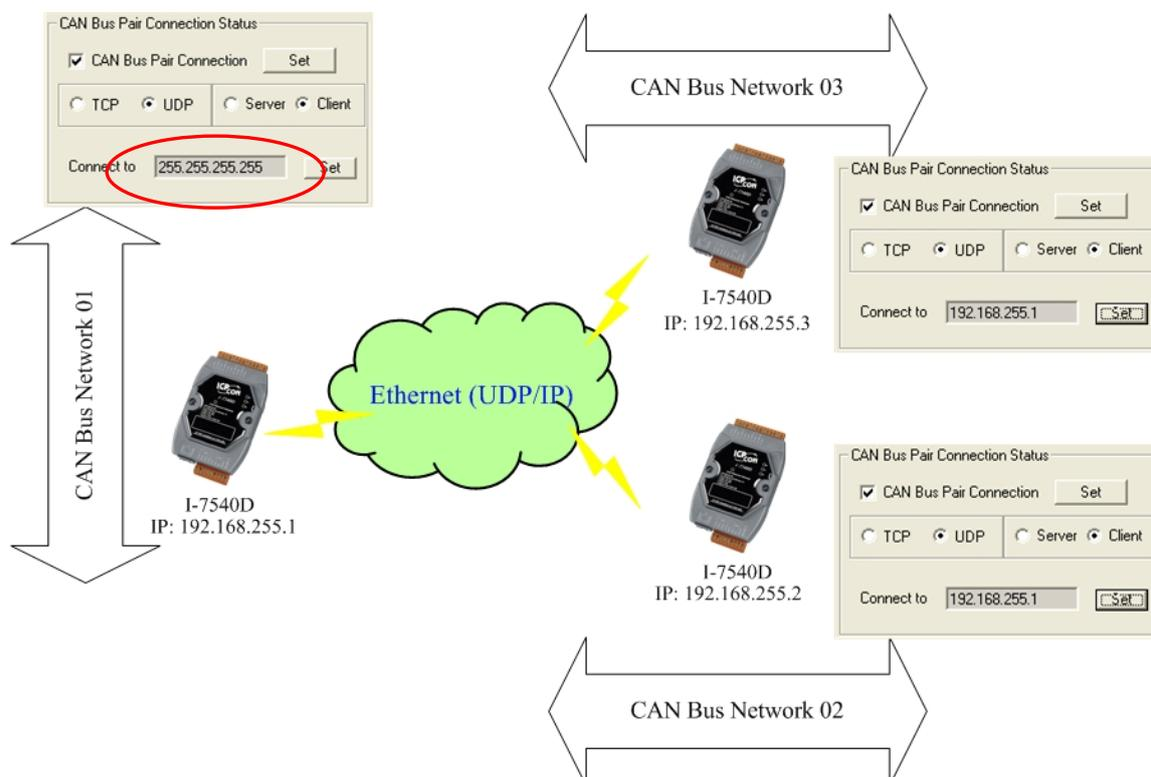
1. After setting “CAN Bus Pair connection Status” of these I-7540D and re-start the system of them, CAN messages on “CAN Network 01” will be sent to “CAN Network 02” and “CAN Network 03” by using UDP/IP protocol via Ethernet network.
