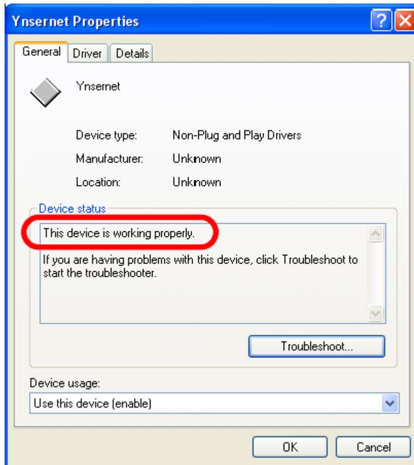
**Problem 3:** The client programs successfully open the COM port, but fail to access the device.
