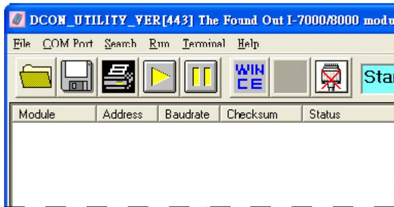
Step 5: If the VxComm Driver works properly, the DCON Utility can search the module(s) connected to COM2 of the I-7540D.
