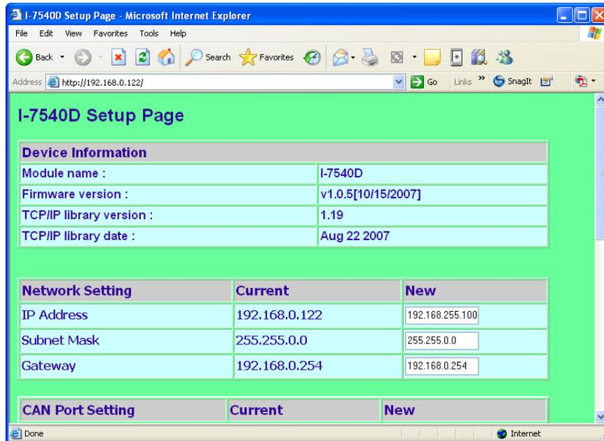
When users want to modify the configuration of I-7540D via Setup web page, they need to fill these two fields, ID and PASSWORD, with correct values. Or they can view the configuration of I-7540D, and can't modify the configuration.
