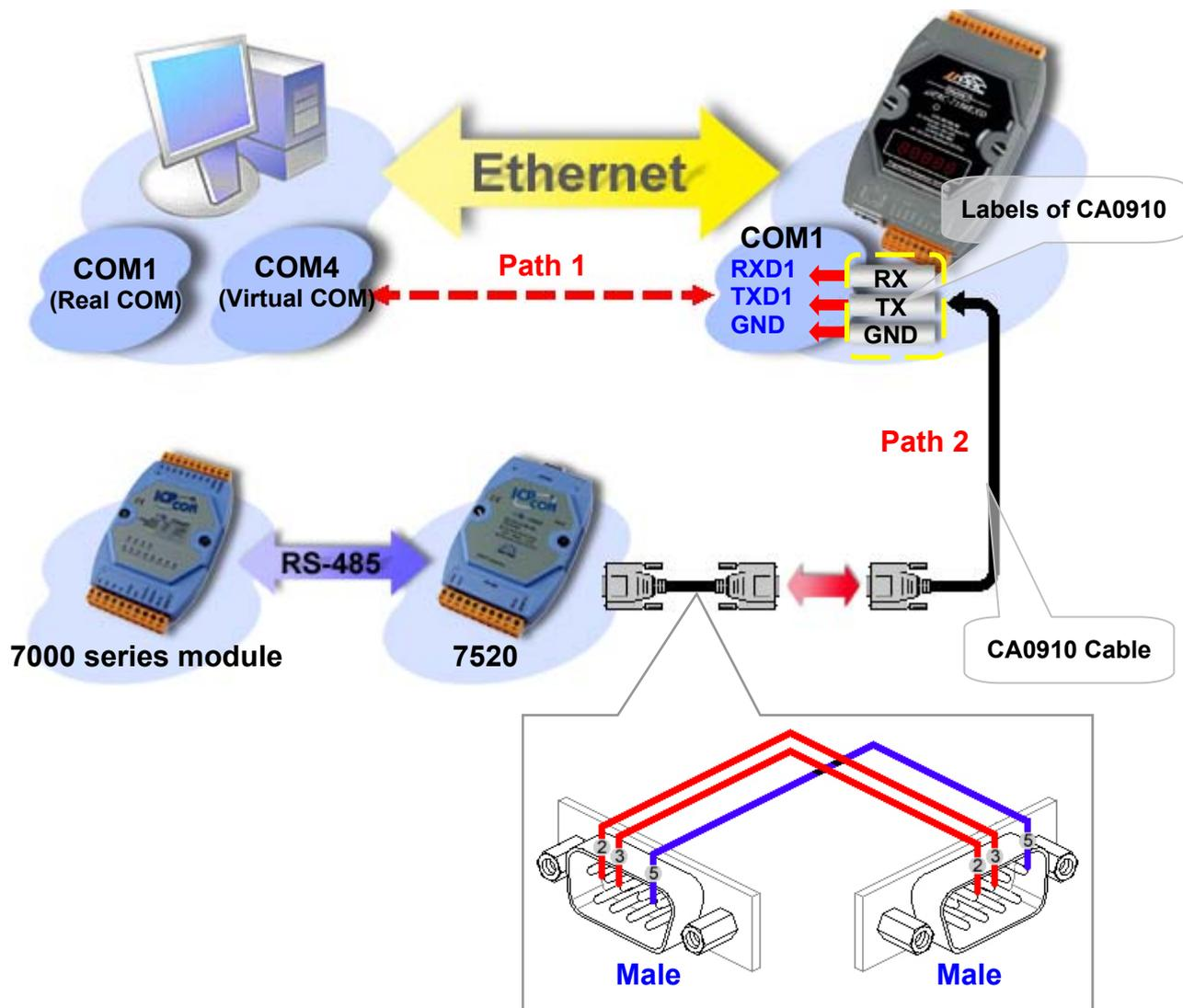
Step 3: Click the COM Port to choose the COM port number, baud rate, and checksum. For example: COM10, 115200, 19200, 9600 and No-Checksum. (These settings depend on the settings of 7000 series module.)
