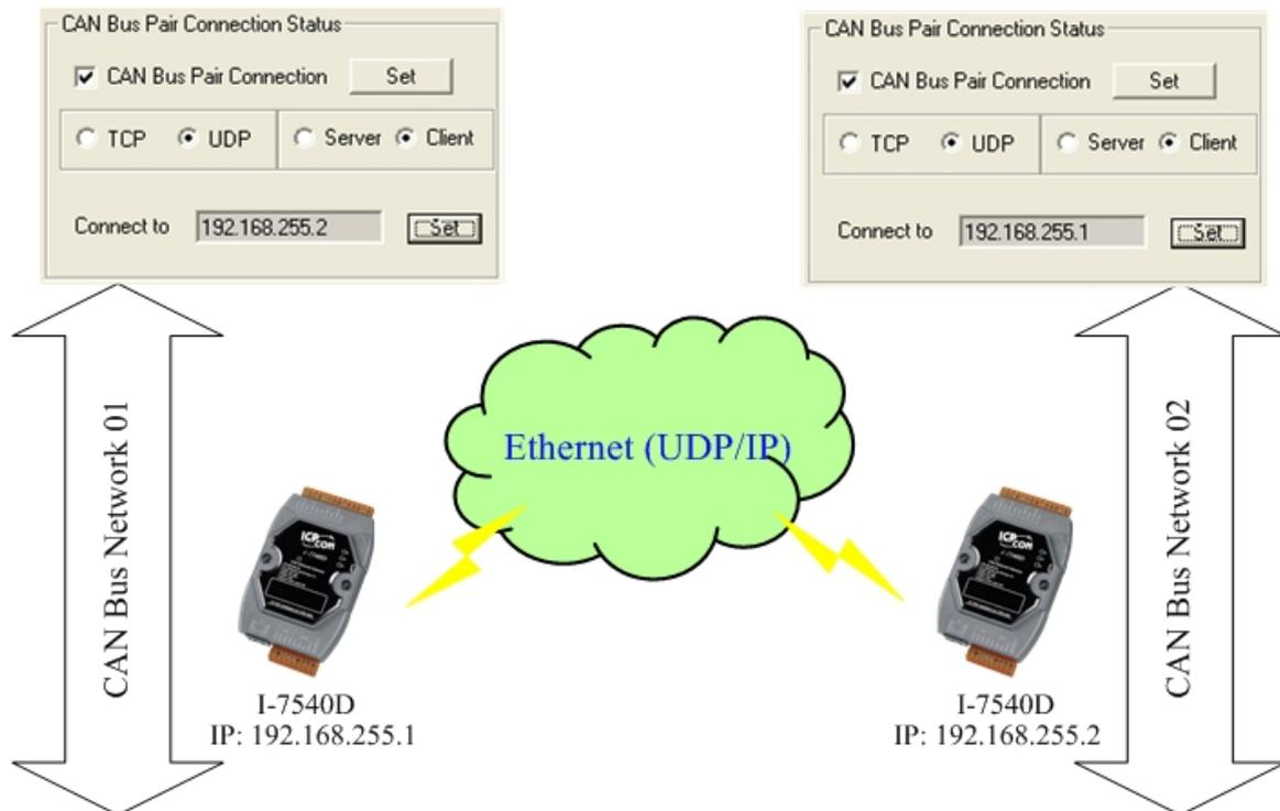
After setting “CAN Bus Pair connection Status” of the two I-7540D and re-start the system of them, CAN messages between “CAN Network 01” and “CAN Network 02” can be exchanged by UDP/IP protocol through Ethernet network.
