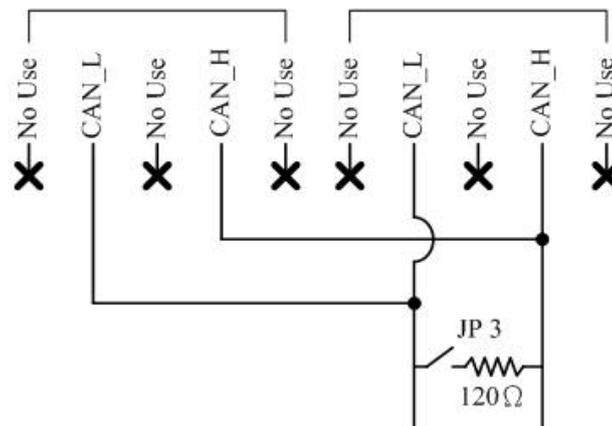
Figure 2-3 Electronic circuit of CAN bus connector
