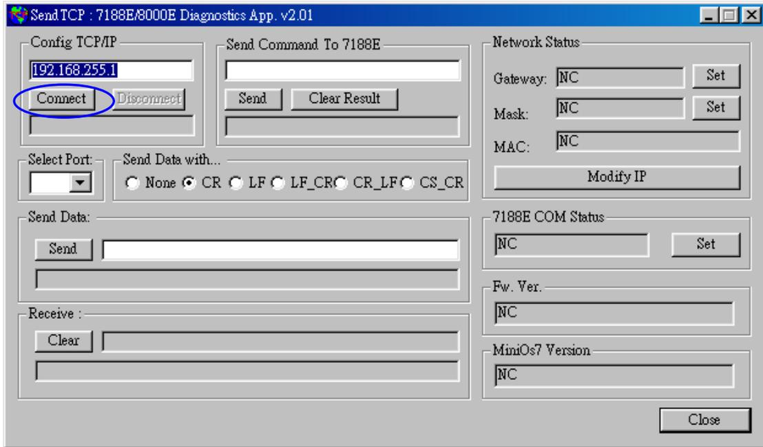
Step 2: Input the IP of I-7540D and press the “**Connect**” button to connect with I-7540D. And then it will display “7188E3 is connected”.
