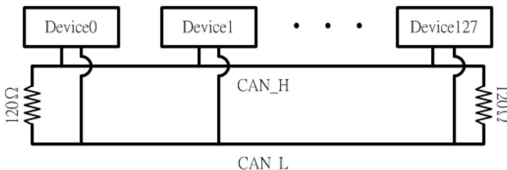
Figure 2-4: Terminator resistor
