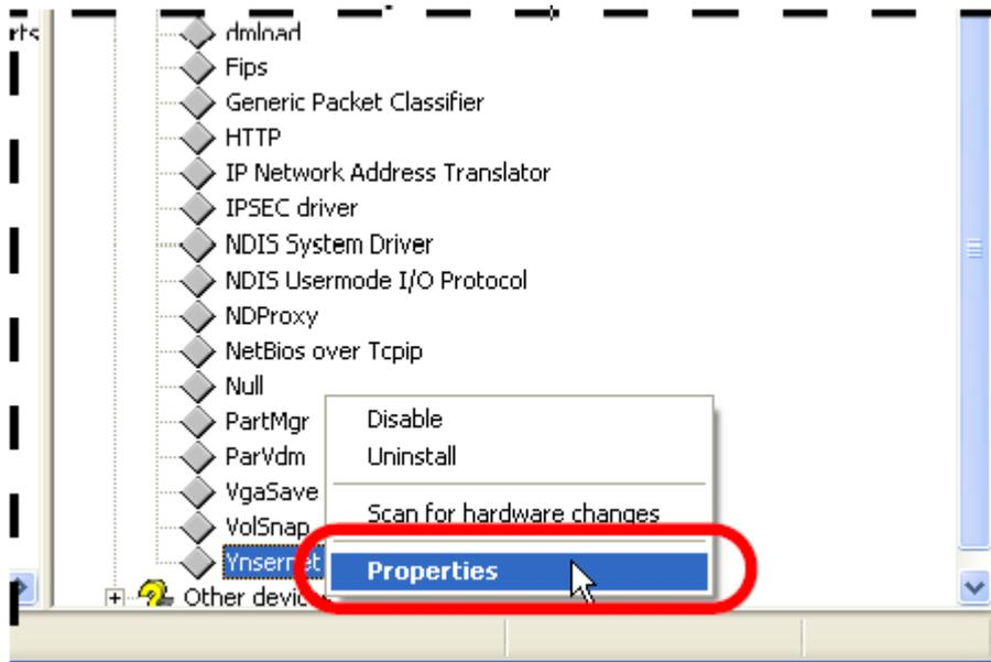
Step 6: Check that the message “This device is working properly” is displayed. If the driver is shown as not working properly, remove it and then re-install and reconfigure the driver.
