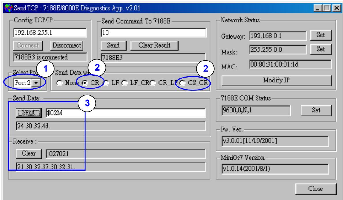
Step 5: If you want to change the 7540D's COM ports settings, click "Set" to change them. The 7540D's COM port that you want to configure is specified by "Select Port" combo list. Port 2 means you want to configure the 7188E's COM2.
