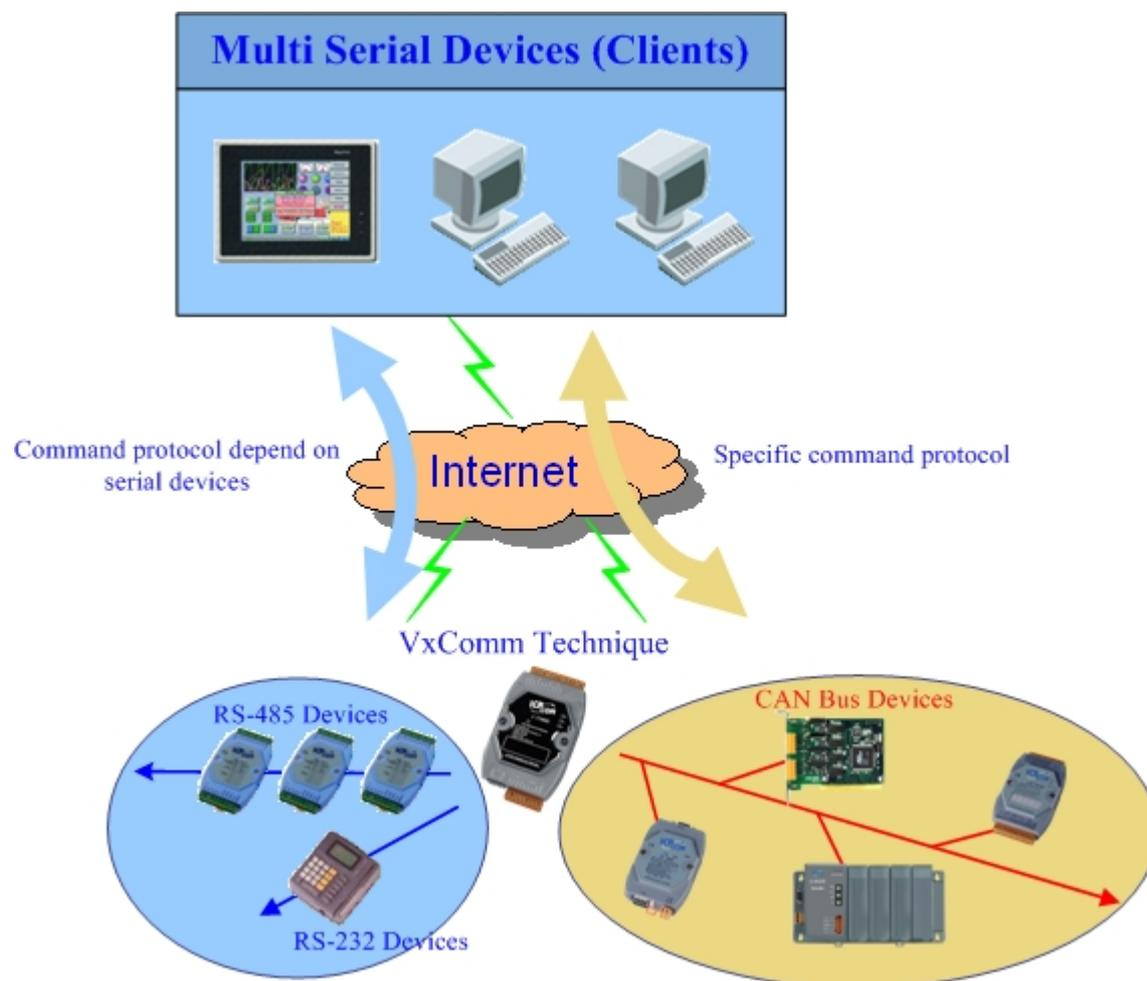
The VxComm technology can be used to simulate COM/CAN ports of the I-7540D to become a COM port of PC. With the help of VxComm driver, users can access the remote COM/CAN ports of the I-7540D just as they would access the PC's COM port.
