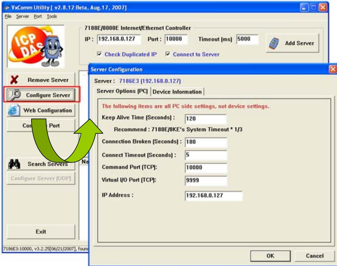
Step 7: Enter the new configuration settings. The new settings will replace any text already in the Server Options window text boxes. Click the **OK** button to save the new settings.
