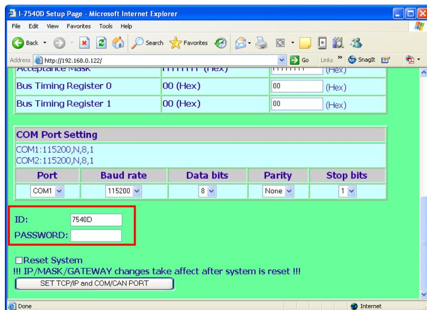
If users want to change the ID and PASSWORD, they need to modify these two parameters by using Utility tool. The default setting of ID is “7540D”, and default PASSWORD is “icpdas7540D”.
