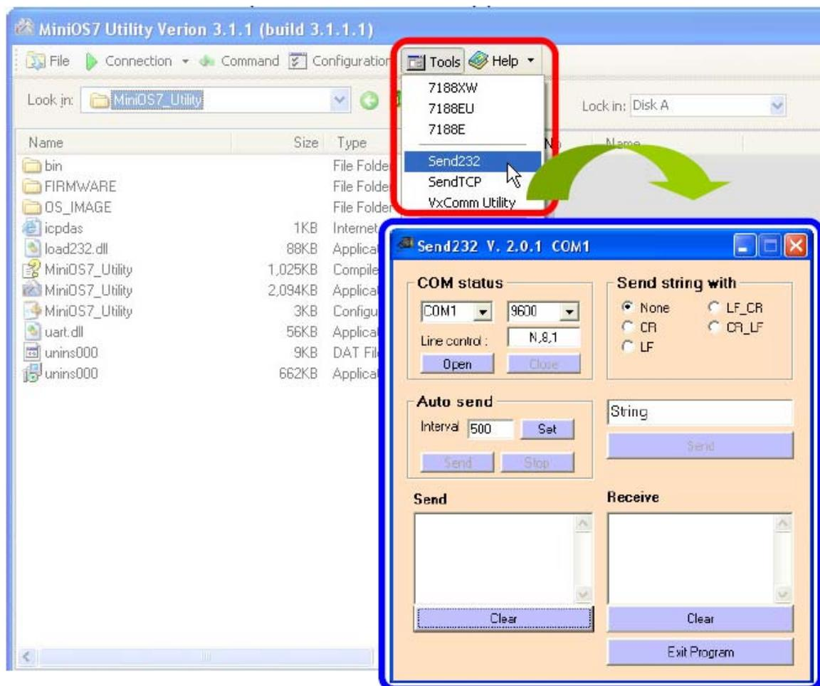
Step 4: Select the COM4, and then click the Open button to open COM4 of the Host PC.
