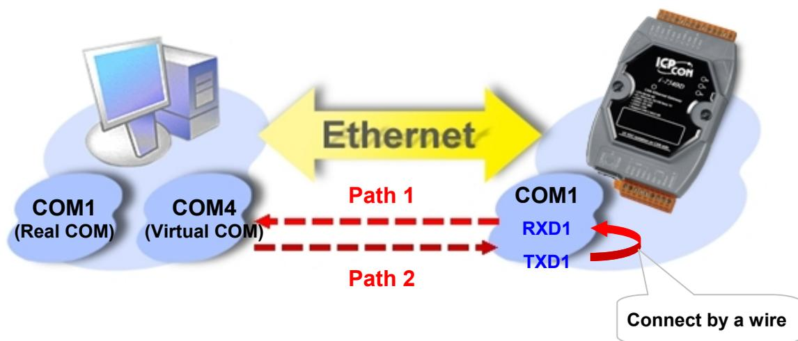
Step 2: Set COM1 of the I-7540D as virtual COM4 of the Host PC using the VxComm Utility.
