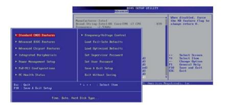
An x86-compatible computer hardware requires a BIOS (Basic Input/Output System) or, more recently, a UEFI (Unified Extensible Firmware Interface). This so-called firmware makes the hardware ready for operation and starts the operating system. Among other things, many hardware functions are activated and configured via the BIOS.
