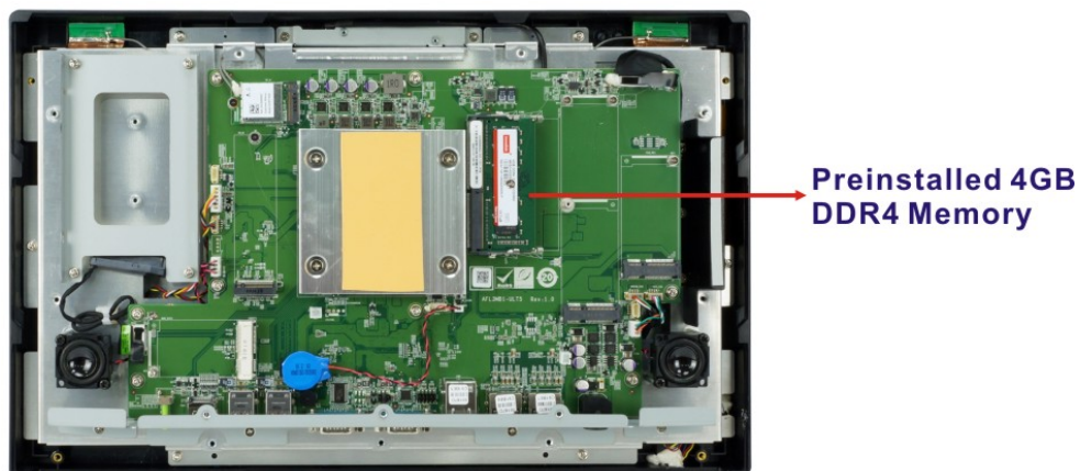
Figure 5-1: SO-DIMM module Location
