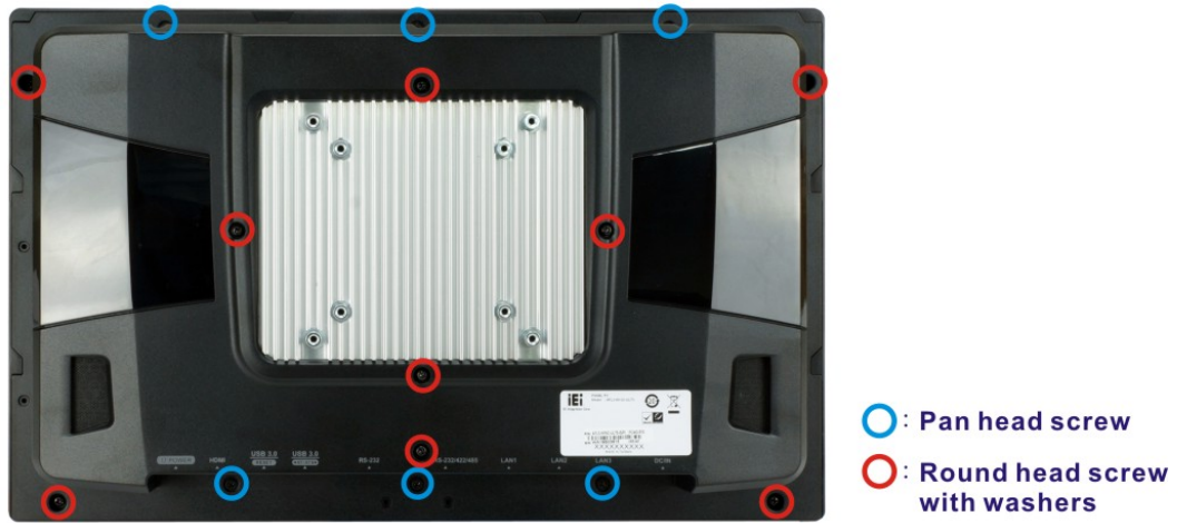
Figure 3-1: AFL3-W15C-ULT5 Back Cover Retention Screws
