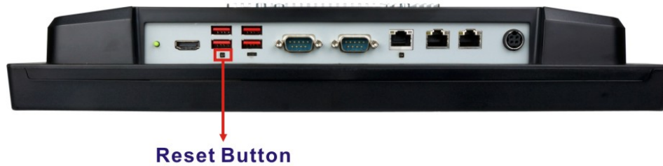
Figure 3-38: Reset Button Location
