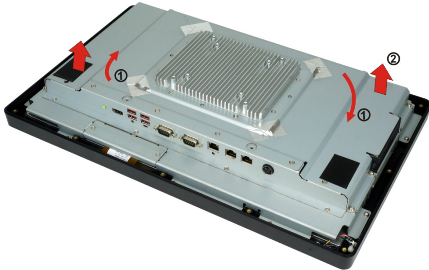
Figure 3-7: Lift the Metal Cover
